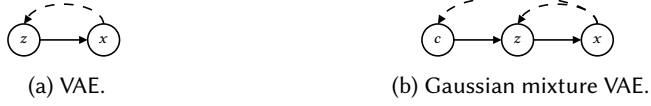
Fig. 15. The traditional VAE and the Gaussian mixture VAE. x is the input, z is the stochastic latent variable, and c is the categorical latent variable. The solid lines depict the generative process, while the dashed lines represent the variational approximation.
