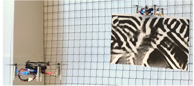
Fig. 1. The attack scenario of this work: a multirotor carries two adversarial patches (printed one per side). The adversarial patches are able to prevent the NN from predicting the relative pose of a human subject in the input image, regardless of the human’s position in the image. Instead, the NN predicts a pose previously chosen by the attacker policy that selects a patch and the relative position of it with respect to the victim.
