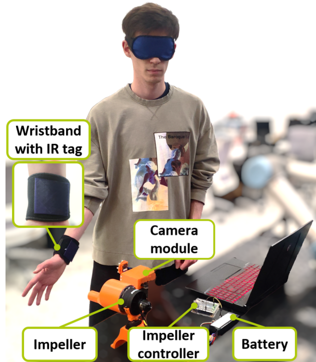
Fig. 4. Experimental setup for measuring the accuracy of the air pressure perception.
