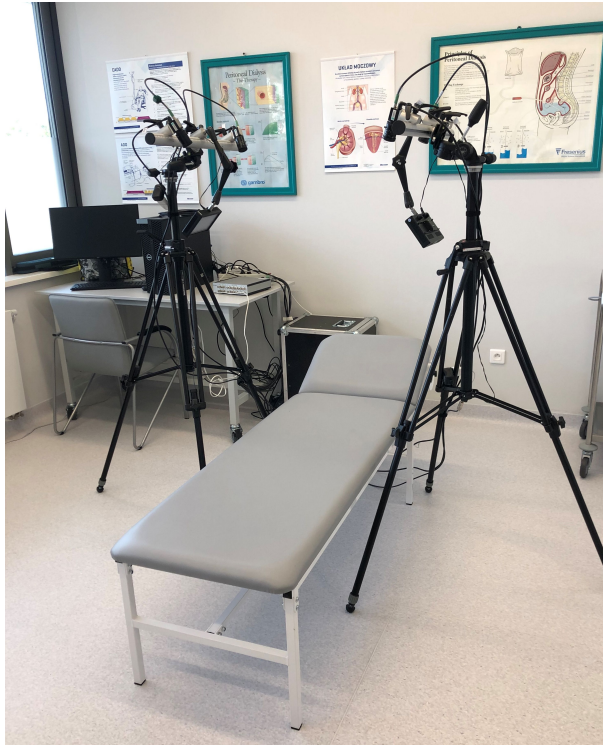
Figure 2: Digital Image Correlation - experimental stand
