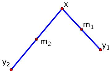
Figure 1. Two-linkage: the no-slip condition is imposed at points  $m_1$  and  $m_2$ .
