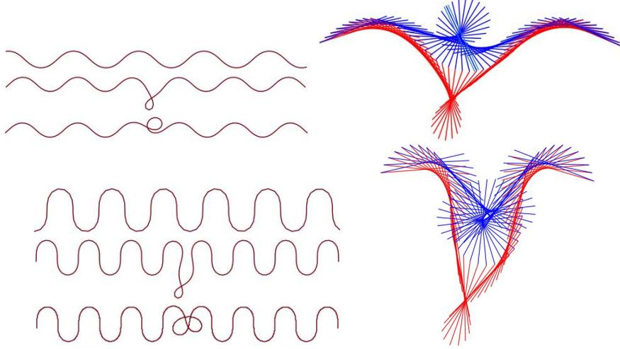
Figure 4. On the left, the trajectories of points  $x, y_1$ , and  $y_2$  are shown, and on the right, the respective motion of the 2-linkage whose two links are colored red and blue. The values of  $k$  are 0.1 and 0.707, respectively.
