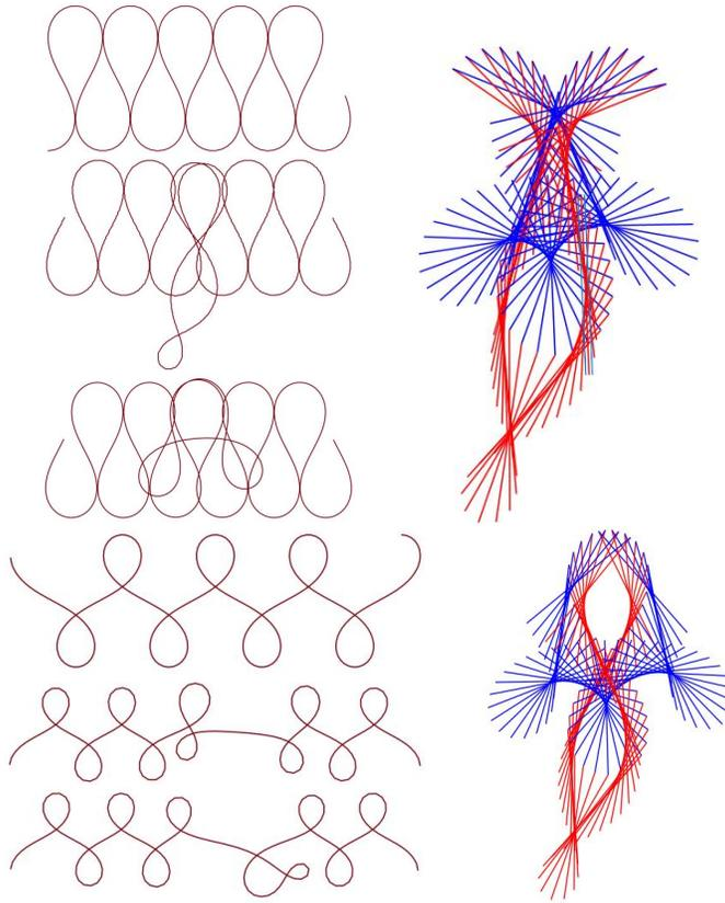
Figure 5. On the left, the trajectories of points  $x, y_1$ , and  $y_2$  are shown, and on the right, the respective motion of the 2-linkage. The values of  $k$  are 0.854 and 0.95, respectively.
