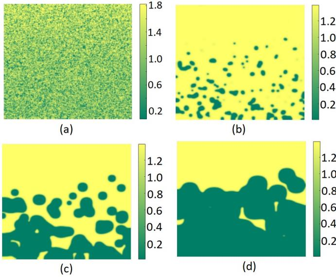
**Fig. 6** Diffusion in two dimensions with positive exponential initial condition. Snapshots are taken after time (a) 12 (b) 225 (c) 1000 (d) 2000. Parameter values are  $\alpha = 13.1$ ,  $\phi = 0.3$ ,  $\lambda = 0.6$ ,  $\delta = 0.01$ ,  $k = 10$ ,  $k_1 = 2$ ,  $k_2 = 0.00001$ . Diffusion coefficient  $D_U = 0.02$ .
