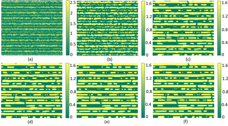
**Fig. 7** Diffusion in two dimensions with stochastic periodic initial condition. Snapshots are taken after time (a) 30 (b) 80 (c) 1350 (d) 2000 (e) 3000 (f) 5000. Diffusion constant is taken as  $D_U = 0.01$ . Rest of the parameter values are  $\alpha = 13.2$ ,  $\phi = 0.3$ ,  $\lambda = 0.6$ ,  $\delta = 0.01$ ,  $k = 10$ ,  $k_1 = 1.5$ ,  $k_2 = 10$ .
