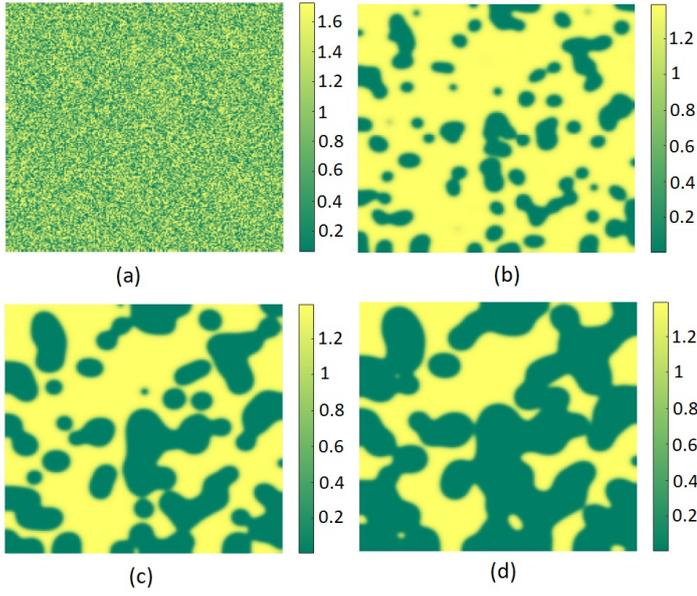
**Fig. 5** Diffusion in two dimensions for randomly distributed initial condition. Parameter values are  $\alpha = 13.1$ ,  $\phi = 0.3$ ,  $\lambda = 0.6$ ,  $\delta = 0.01$ ,  $k = 10$ ,  $k_1 = 1.8$ . Diffusion coefficient  $D_U$  is taken as 0.05. Snapshots are taken after time (a) 1 (b) 250 (c) 500 (d) 700.
