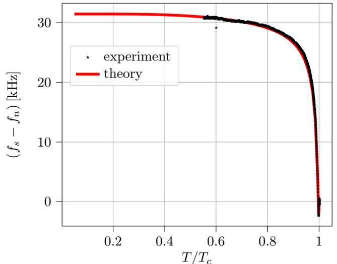
FIG. 2 The frequency shift  $\delta f = f_s - f_n$  as a function of temperature for a cavity with fundamental frequency  $f = 2.6\text{GHz}$ . The data (black symbols) are from Ref. /onlinecitebaf21. The theoretical result (red line), based on Eqs. (9) and (4), corresponds to a quasiparticle scattering rate of  $\tau = 0.257\text{ps}$ . Note the negative shift close to  $T_c$ .
