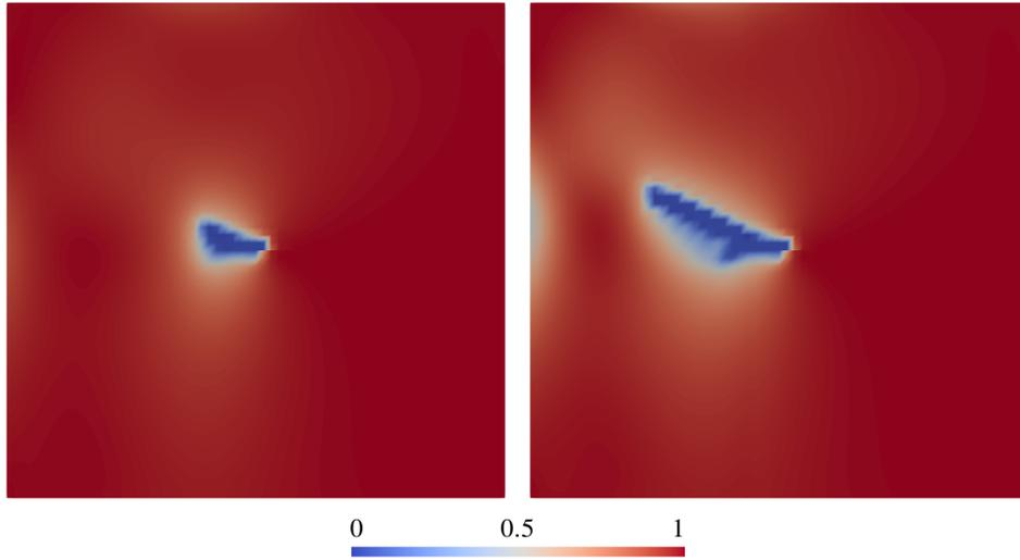
FIGURE 6.1. Crack Pattern of Example 1 after 500 timesteps for initial control (left) and final control (right) on a  $64 \times 64$  mesh
