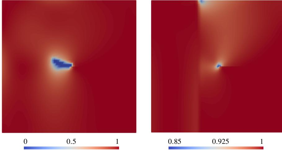
FIGURE 6.3. Crack Pattern of Example 2 after 100 timesteps for initial control (left) and final control (right) on a  $64 \times 64$  mesh
