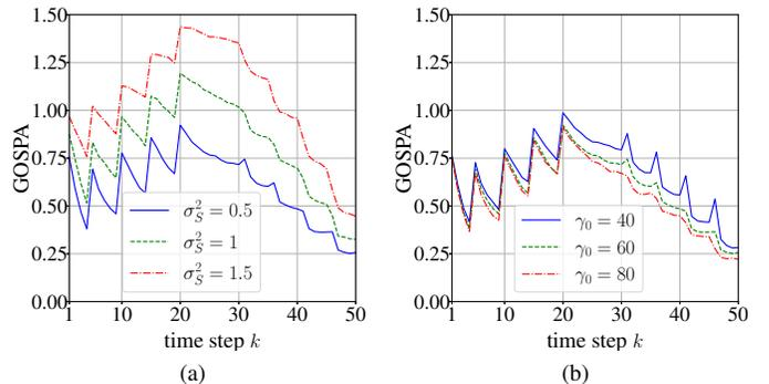
Fig. 3: GOSPA metric the proposed TBD-BP ( $L = 2$ ) with (a)  $\gamma_0 = 60$  and different  $\sigma_S^2$ ; (b)  $\sigma_S^2 = 0.5$  and different  $\gamma_0$ .
