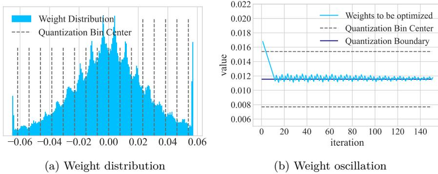
Figure 4: The visualization of weight distribution during quantization-aware training and the weight oscillation effect due to distribution variance. The layer we select is *blocks.1.attn.proj-v.weight* in 4-bit quantized DeiT-S with scale  $\alpha = 0.0077$ .
