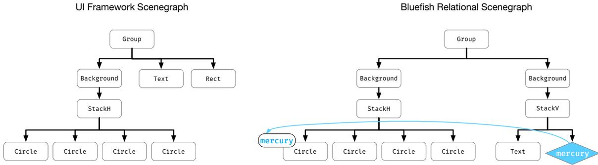
**Figure 5: The tree-structured and relational scenegrphs corresponding to Figure 2. Notice that Bluefish’s scenegrph retains more information than a tree-structured scenegrph. Bluefish’s scenegrph represents the `StackV` and `Background` relations between the label and the planet. In the traditional scenegrph the `StackV` relation between the label and the planet is missing, and the `Background` relation has been reduced to a `Rect` component.**
