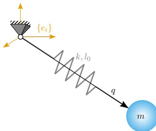
Figure 1: Spring pendulum system with orthonormal basis  $\{e_i\}$ .
