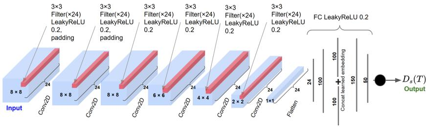
**Figure 4.** *Spatial discriminator  $D_s$  architecture. The inputs to the spatial discriminator  $D_s$ , are the  $8 \times 8 \times 24$  temperature maps. The input is then passed through a series 2D convolution layers with the output of the prior layer serving as input into the following layer. The final convolution layer outputs a 2-dimensional  $24 \times 1$  vector, which is flattened into a one-dimensional vector before it is passed through a dense FC linear block to produce a score.*
