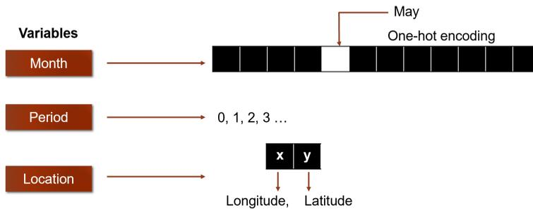
**Figure 14.** Each conditional variable is passed into a model block that transforms it into a higher dimensional learned embedding, resulting in the labels being mapped from  $\mathbb{R}^{15}$  to  $\mathbb{R}^{100}$ .
