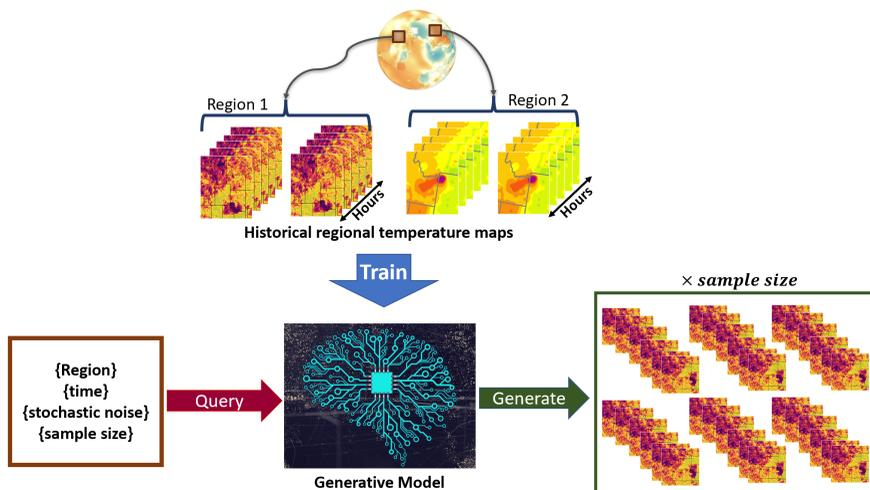
**Figure 1.** *TemperatureGAN model framework. Regional temperature maps are passed as input to discriminator during the training, however the generator never sees the training data.*
