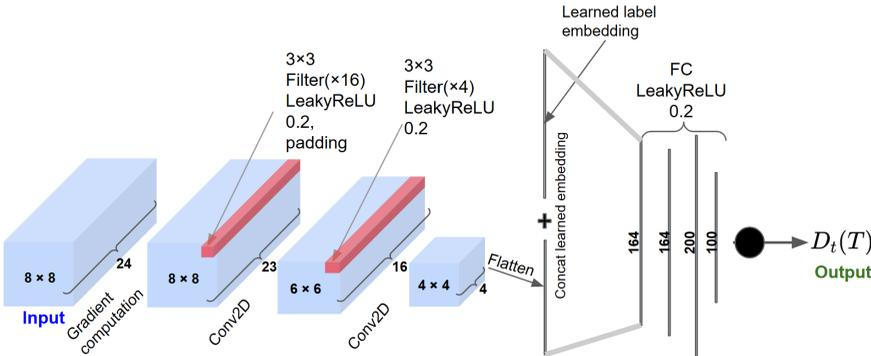
**Figure 5.** *Temporal discriminator  $D_t$  architecture. The inputs to the temporal discriminator  $D_t$ , are the  $8 \times 8 \times 24$  temperature maps and then a gradient computation is followed, to compute  $\frac{\partial T}{\partial t}$ . The output from the convolution layers is flattened and passed through a series of fully-connected (FC) linear layers to produce a score.*
