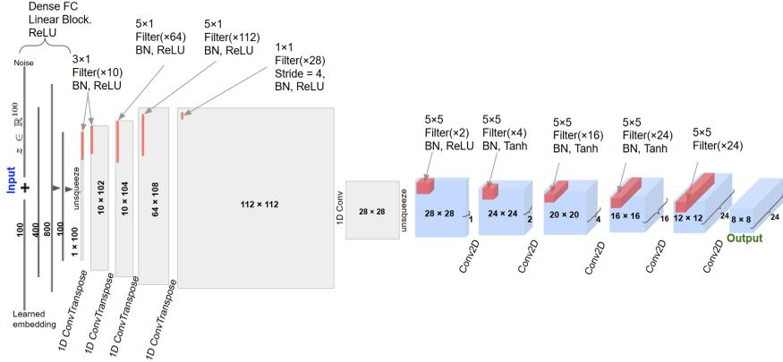
**Figure 3.** *Generator  $G$  architecture. The sampled noise is concatenated with the learned label embedding and passed through a dense, fully-connected (FC) linear block with Rectified Linear Unit (ReLU) activation functions. The output of the linear block is sent through series of convolution layers with batch normalization to obtain the desired  $(8 \times 8 \times 24)$  output shape.*
