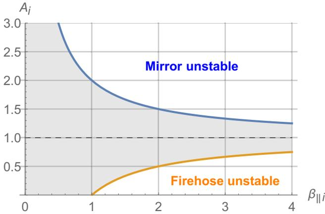
**Figure 3.** Stability diagram. The plasma is stable within the shaded area.
