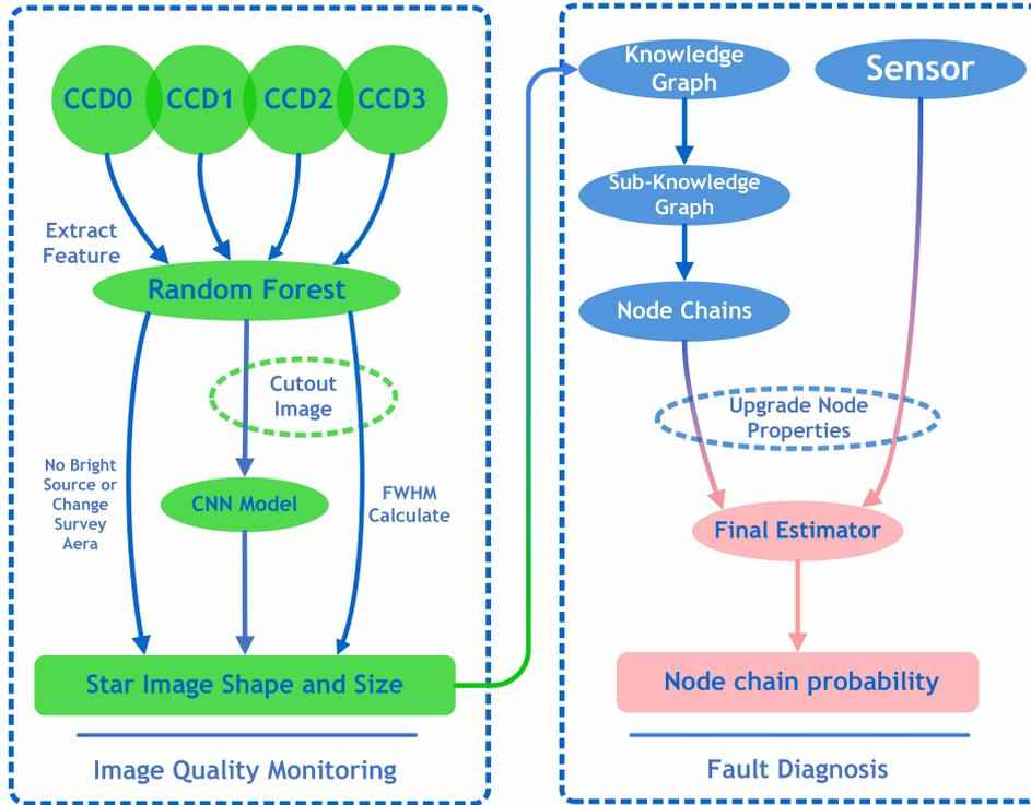
**Fig. 6** In the framework of the telescope maintenance support system, the left part realizes the imaging quality monitoring, and the right part realizes the fault diagnosis(Hu et al., 2023)
