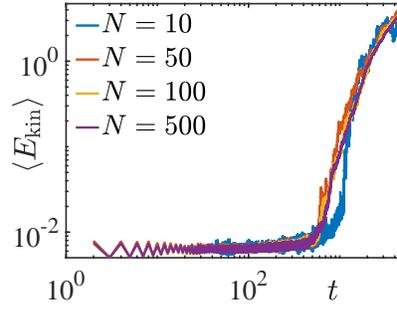
FIG. S4: Time evolution of the averaged kinetic energy for the TM drive. The simulation results converge for large systems and  $N = 500$  is already sufficient to produce thermodynamically large systems. Here we use the kick strength  $K = 0.07$  and the results are averaged over 200 random realizations. Initial states are the same as in Fig. 1.
