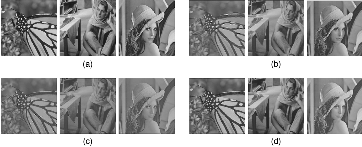
Fig. 5: Effects of embedding watermarks by using CA-QIM over different lattices. (a) Original image (b) \Lambda_f = A_2 (c) \Lambda_f = D_4 (d) \Lambda_f = E_8 .
