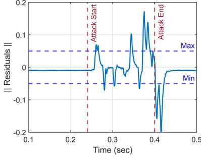
Fig. 2. Response of the SKR event detection scheme during a control input attack targeting DG inverter controller.
