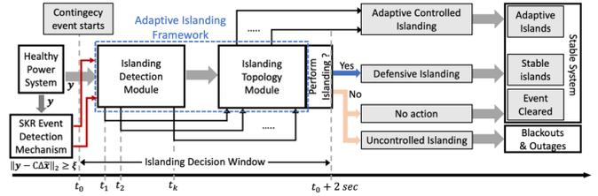
Fig. 1. Overview of the event-triggered islanding framework.
