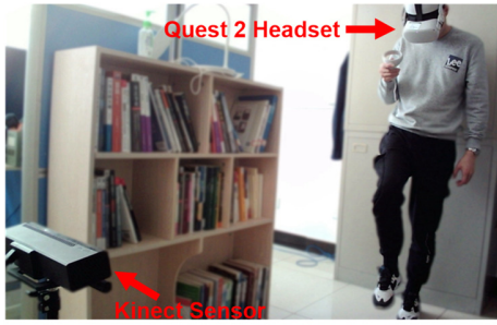
Fig. 3. Experimental Setup. Demonstration by a researcher, performing in-place walking with movements captured by a Kinect v2 sensor.
