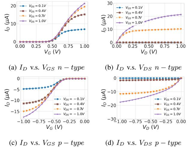
Fig. 2: Characteristics of MIV-transistor
