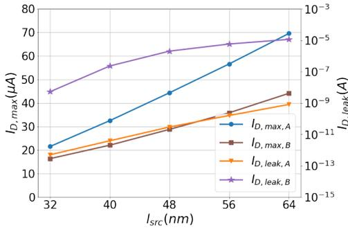
Fig. 3:  $I_{D,max}$  and  $I_{D,leak}$  v.s.  $l_{src}$
