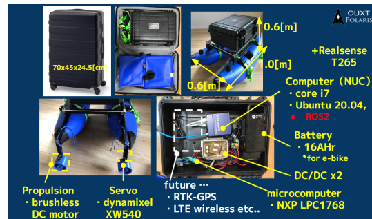
Fig. 10. Hardware Components of MINI-V
