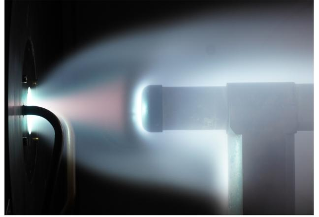
Figure 2: Schematic of the inductive plasma generator IPG4 (left) and photograph of its CO<sub>2</sub> plasma plume during heat flux measurements at  $\dot{m}_{\text{CO}_2} = 2.2 \text{ g/s}$ ,  $P_A = 160 \text{ kW}$  and  $p_{\text{amb}} = 100 \text{ Pa}$  in PWK3 (right).
