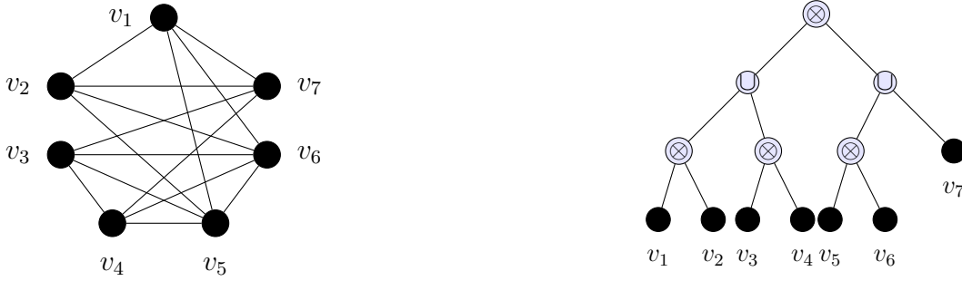
FIGURE 1. A cograph G = ((v_1 \otimes v_2) \cup (v_3 \otimes v_4)) \otimes ((v_5 \otimes v_6) \cup v_7) and its cotree T_G .
