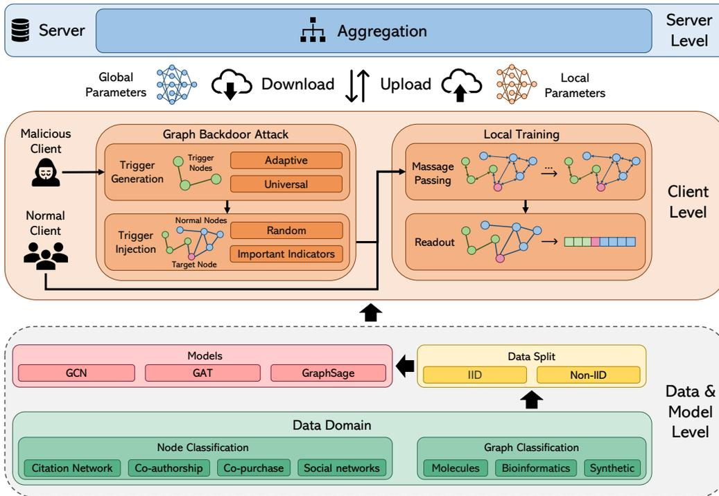
Figure 1: A unified framework for classification backdoor attack on FedGNN.
