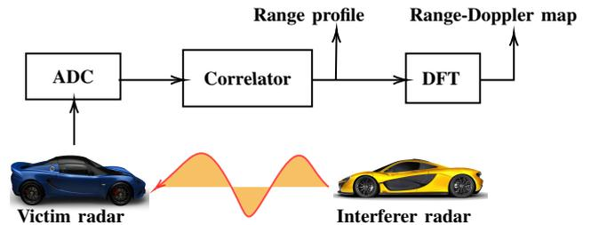
Fig. 1: A simplified illustration of the PMCW radar operation and PMCW-PMCW mutual interference between two vehicles.
