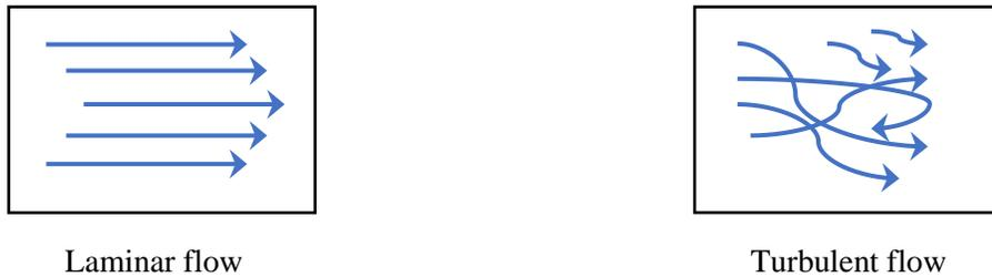
**Figure 1.** Laminar and turbulent flows.
