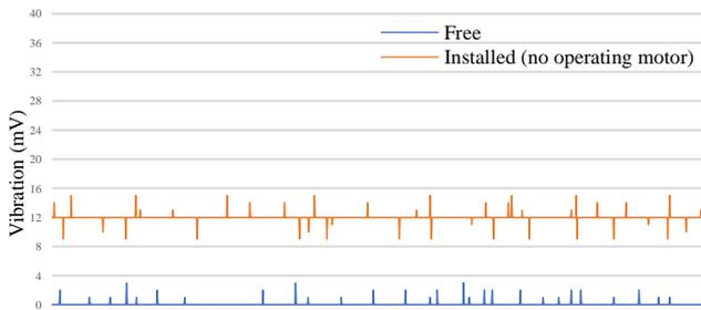
Figure 3. Test apparatus vibration in the free state
