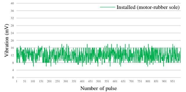
Figure 5. Test apparatus vibration when using a rubber sole
