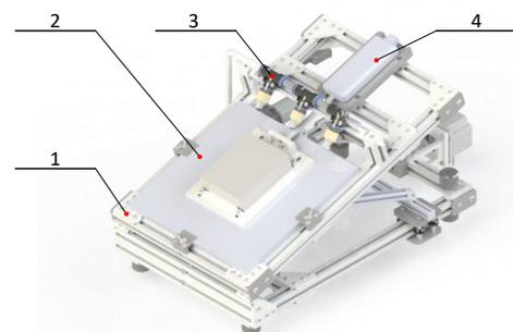
Figure 1. 3D design of the slip resistance test apparatus
