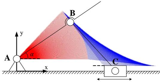
Figure 2. Kinematic diagram and operating simulation of the slip resistance test apparatus
