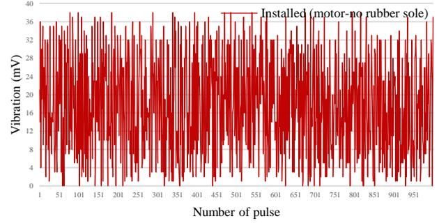
Figure 4. Test apparatus vibration when the rubber sole is not used
