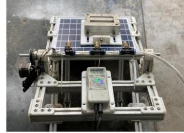
Figure 10. Actual image of test apparatus, slip detection at 29.3°
