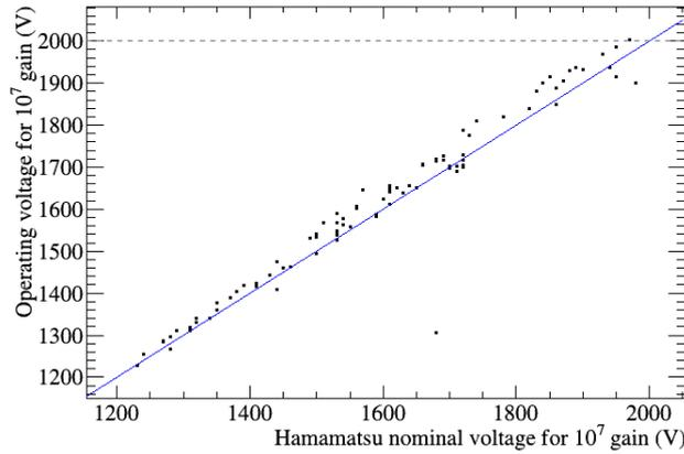
**Figure 6:** Comparison of calculated operating voltages with Hamamatsu nominal voltages for  $10^7$  gain from full fits to filtered histograms. The grey dashed line represents the maximum operating voltage of 2000 V. The outlier has been put down to an error in the shipping data.
