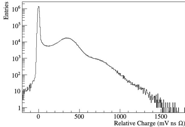
**Figure 4:** Typical relative charge spectrum with a pedestal peak at  $\sim 0$  mV ns  $\Omega$ , a single-photoelectron peak at  $\sim 400$  mV ns  $\Omega$  and later multiple-photoelectron peaks in the tail.
