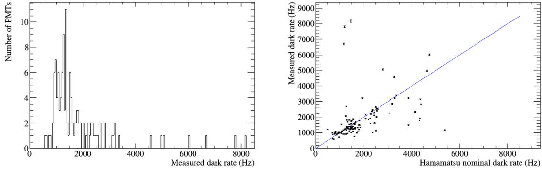
**Figure 8:** Results of the dark rate tests showing the distribution of measured dark rate distribution in 50 Hz bins for all PMTs tested (left) and the measured dark rates compared to the Hamamatsu nominal dark rates (right).
