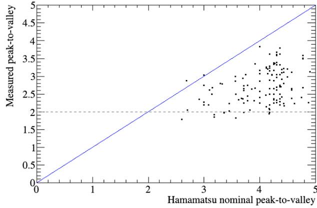
**Figure 7:** Measured peak-to-valley measurements, versus the Hamamatsu data sheet values. The grey dashed line shows a potential requirement of a peak-to-valley ratio of 2. Errors on the values (not visible) are between 0.01-0.02 (absolute uncertainty).
