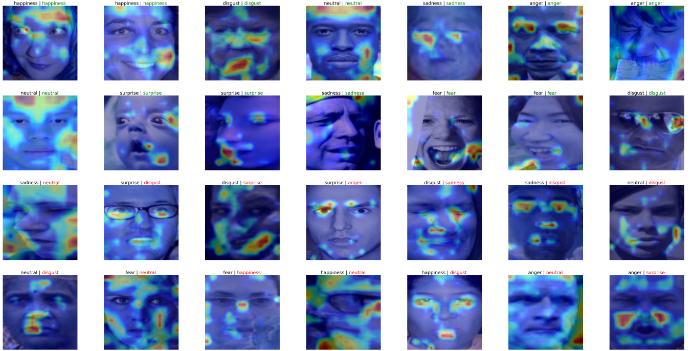
FIGURE 7. Examples of true and false predictions on RAF-DB and their activation maps. The ground truths of the samples are labeled in black whereas the true and false predictions are labeled in green and red, respectively.
