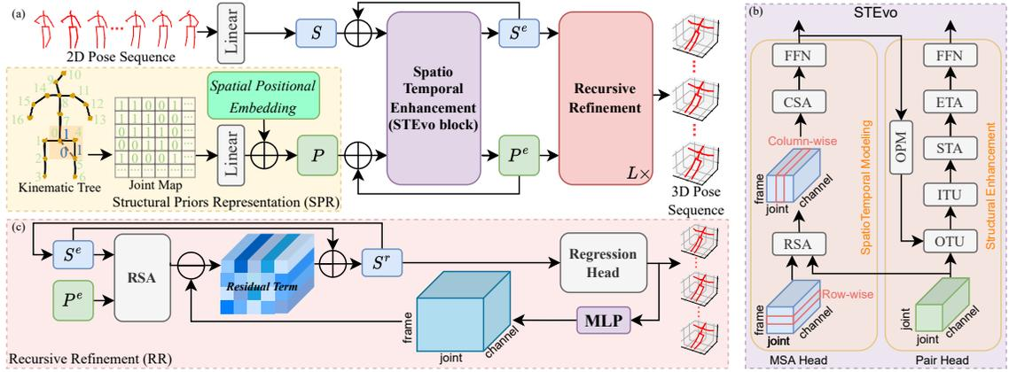
**Fig. 1:** (a) Overview of the proposed EvoPose. Structural Priors Representation (SPR) derives structural features from the kinematic tree. SpatioTemporal Enhancement (STE) models spatiotemporal relations and enhances structural features. (b) Overview of STEvo in STE. (c) Overview of the Recursive Refinement (RR) which refines the estimated result auto-regressively.
