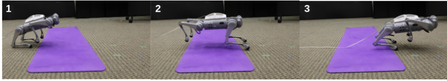
Figure 4: Using the bounding gait, the robot can jump over a 60cm-wide yoga mat without making foot contact.
