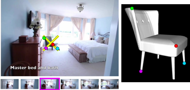
Figure 3. We ask humans to annotate point correspondences between the 3D surface of the CAD model and the video frames of the tracked object.
