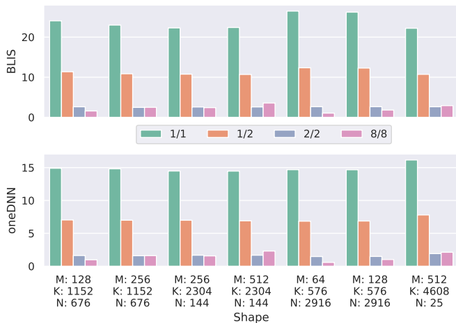
Fig. 5. Comparison between matrix multiplication routines at different quantization levels. M is the number of rows of the first operand, K is the shared dimension, and N is the number of columns of the second operand.
