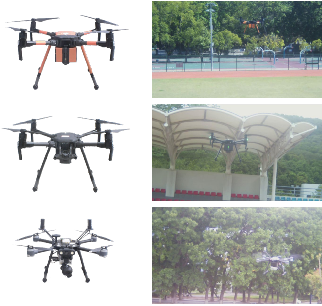
Fig. 9. The illustration of different target UAVs. From top to bottom is M200 Orange, M200 black and P600, respectively. Best viewed in color.
