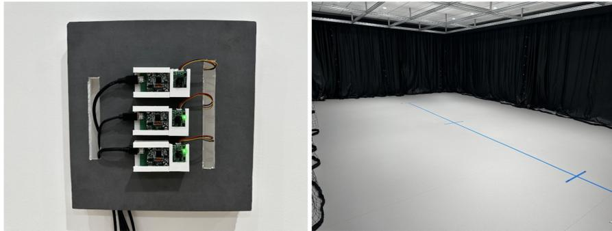
Fig. 7. This figure presents a dual-view illustration. The left panel shows a wall-mounted sensor assembly, consisting of sensors developed in-house the left side and those provided by a commercial partner on the right. The right panel depicts the experimental environment where study participants stood in front of the sensor setup. Distances from the sensor setup (1m, 3m, and 5m) are marked on the floor for participant positioning.
