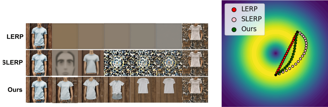
Figure 1: The interplay between interpolation and input distribution. (Left) Visual comparison of three interpolation methods between a pair of seeds in the high-dimensional space of Stable Diffusion [46]. Interpolation paths computed by linear (LERP) and spherical SLERP [56] interpolation produce seeds that result in images that are flat or just noise, whereas our approach is capable of generating images that are meaningful (quantified in Table 1). (Right) Paths found using linear (LERP), spherical (SLERP), and likelihood-based interpolation methods in 2D space, where the norm of samples has a \chi distribution. Colors denote the log of the probability distribution function. The interpolation path computed by NAO traverses areas that have the desired norm (yellow, high likelihood).
