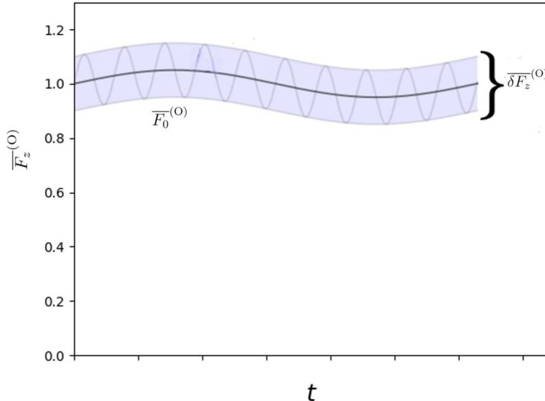
**Figure 1.** Schematic picture describing the equilibrium orbit averaged distribution function  $\overline{F}_z^{(0)}$ . The solid line represents the slowly varying component of the orbit averaged distribution function, while the oscillation around it corresponds to  $\overline{\delta F}_z^{(0)}$ .
