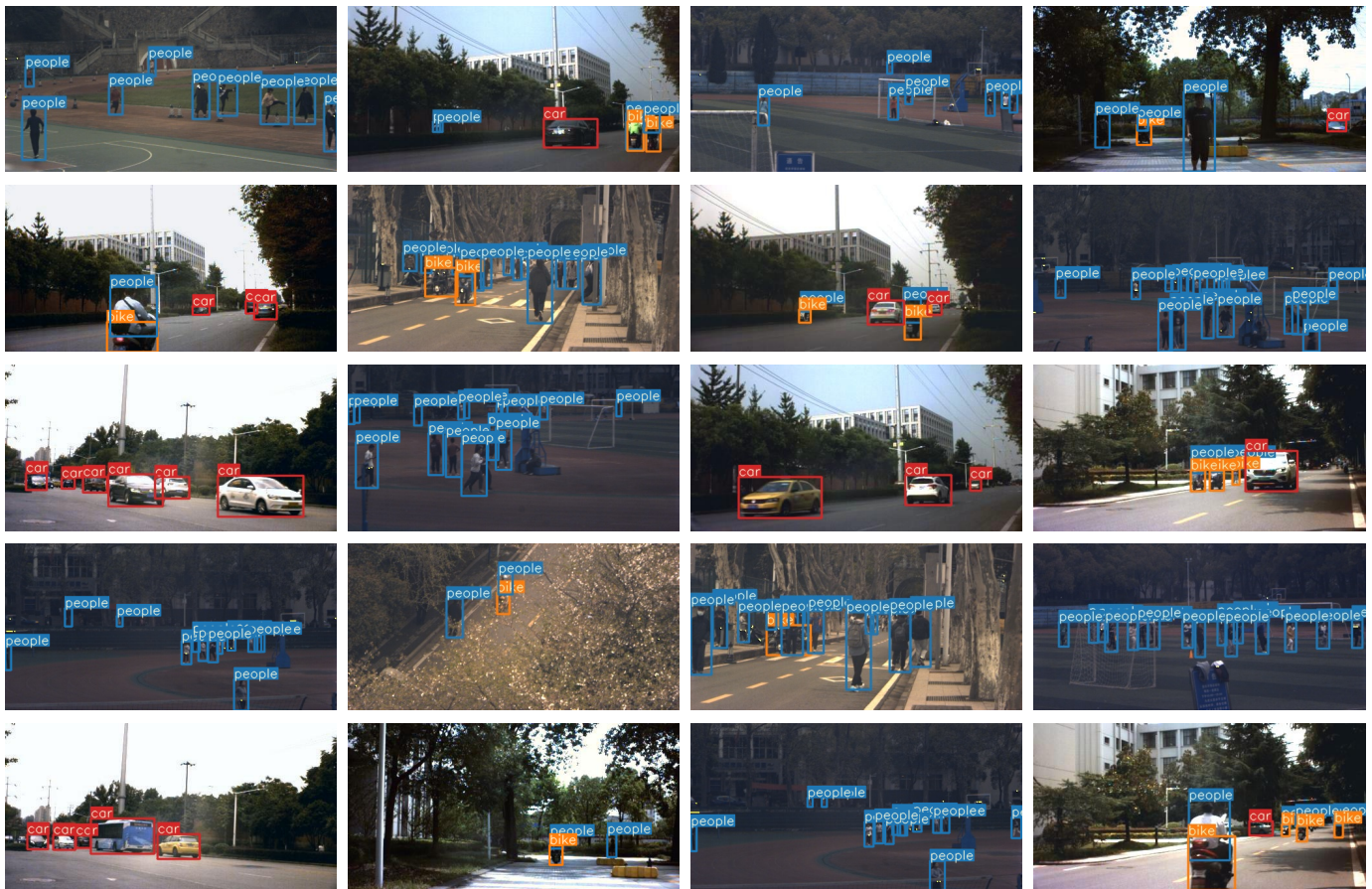
Fig. 6. Visualize some object detection results. The categories of people, bikes, and cars are represented by blue, yellow, and red boxes, respectively. We transformed the hyperspectral images into pseudo-color images for display.
