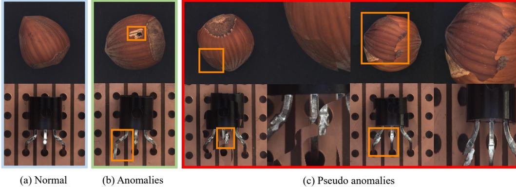
Figure 5. Visualization of normal samples, real anomaly samples and pseudo anomaly samples generated by SaliencyCut from Hazelnut and Transistor of MVTEC AD dataset [3]. (a) and (b) show normal and anomaly samples, respectively. Pseudo anomalies generated by SaliencyCut are presented in (c).
