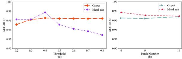
Figure 7. Sensitivity analysis of threshold (left) and patch number (right) on Carpet and Metal\_nut under the hard setting.
