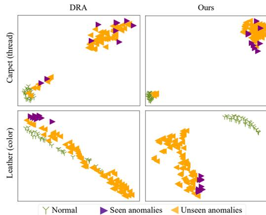
Figure 6. t-SNE visualization of features learned by DRA [7] and our approach during testing on two data subsets of MVTEC AD [3] (Leather and Carpet) under the hard setting. Thread and color are two seen anomaly types during training, respectively.
