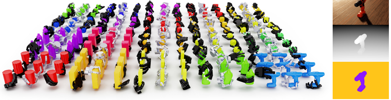
Fig. 1: The Grasp'D-1M dataset contains one million unique grasps, each with multi-modal visual inputs for training vision-based robotic grasping. We synthesize these grasps with a new differentiable grasping simulator, Fast-Grasp'D . Gradient information accelerates the grasp search, allowing us to search the full-DOF space (without eigengrasps) and simulate thousands of contacts to produce a dataset of contact-rich, stable grasps that can improve any learned grasping pipeline.
