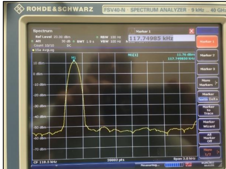
Figure 4. The RCB output for a frequency scan across the bridge resonant frequency with a 100\text{mV}_{\text{rms}} excitation input and \sim 100\text{ fF} differential capacitance. Scan: 117 kHz to 120 kHz (0.3 kHz/division)
