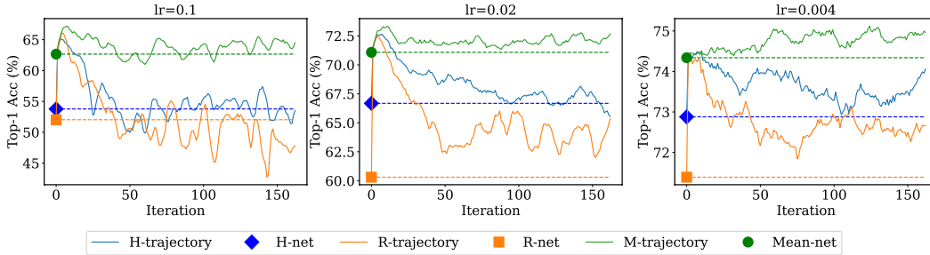
Figure 6: Accuracy curve of sub-model state update on the test set with different learning rates using ResNet50 on CIFAR100. At position 0 on the horizontal axis, H-net (trained by randomly horizontally flipped data) and R-net (trained by RandAugment data) are averaged to Mean-net. Subsequently, during 160 weight iterations, H-net and R-net continue to be trained with their respective data, while Mean-net represents the model obtained by averaging the weights at each iteration.
