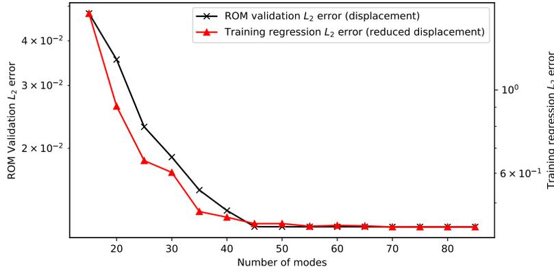
Figure 14: Testing error of the ROM results  $\epsilon$  and the regression error on the training data  $\epsilon_{regression}$  depending on the number of forces modes. Case of the parametric ROM 4.
