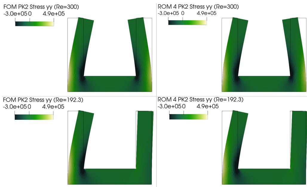
Figure 16: The ROM-FOM (using **ROM 4**) results compared to the FOM-FOM results. This is taken at  $t = 5.84$  s. The  $yy$  component of the PK2 stress field is showed while also showing the complete solid deformation.
