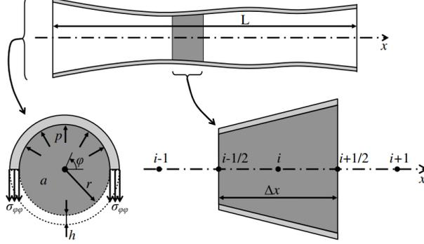
Figure 2: Arterial vessel test case schematic explanation (from [16]).  $\sigma_{\varphi\varphi}$  is the vessel hoop stress,  $h$  is the thickness and  $\Delta x$  is the length of the finite volume cell.
