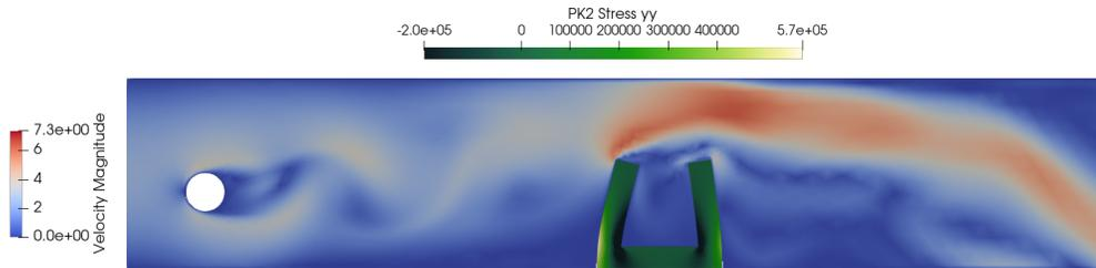
Figure 12: Problem solution at  $Re = 300$  and  $t = 3.62$  s. The velocity magnitude is plotted in the fluid domain, while the  $yy$  component of the second Piola Kirchoff stress (PK2) is showed in the solid domain.
