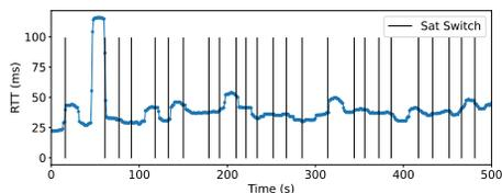
(b) **Sustained Latency Spikes are Not Always Satellite Changes**—Satellite switches are computed using the obstruction map above.
