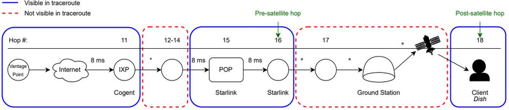
Fig. 3. **Truncated “Outside-In” Traceroute From Public Server to Starlink Dish**—The LEO link is traversed between the last hop and the second-to-last responsive hop, as indicated by a jump in latency.
