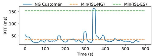
Fig. 10. **ISL Impact On Latency Spikes**—Customer  $e$  located in Nigeria experiences spikes in latency that coincide with the expected latency of different ISL routing methods. We describe the different ISL routing methods in Section 7.2.
