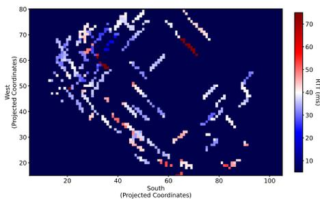
(a) **Sustained Latency Spikes are Not Correlated With Satellite Location**—An image projection of the satellites the dish connects to when facing the sky (Appendix D), overlaid by the user’s RTT when connected to each satellite’s location, shows no correlation between high RTTs and satellite location.
