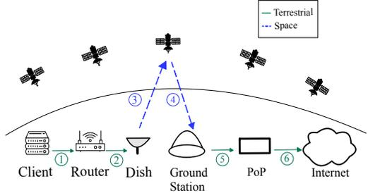
Fig. 2. **Simplified LEO Satellite Network Routing (Egress)**—When a LEO client sends a packet to the public Internet, the packet is sent to a satellite using a dish, and is received by a ground station before forwarding to a POP.
