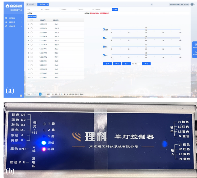
Fig. 2. (a) shows a screen shot of dimming system software (single light control); (b) is the LED road lamp intelligent control dimming hardware module.
