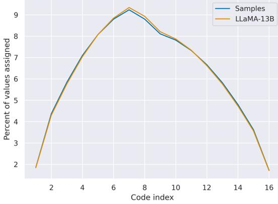
Figure 4: Usage of each NF4 code value for (a) Samples from the generative process in Equation 1 (b) Weights from the LLaMA-13B model. (Quantization block size  $B = 64$ )
