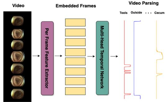
Figure 2. The two stage video parsing pipeline. The first stage is a single frame encoder. The second stage runs temporal convolution (MS-TCN, ASFormer) on frame embeddings to yield per-frame classifications.
