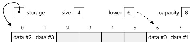
Fig. 5. The storage area is used in a circular fashion, from left to right. The variable lower is used to locate the internal index of data #0 .
