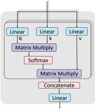
Figure 1: Illustration of self-attention.  $q$ ,  $k$ , and  $v$  denote the query, key, and value, respectively. “Linear” denotes the fully connected neural network layers. For multi-head self-attention, each black box denotes one head and gives a representation. All the representations are concatenated through the concatenate layer and input into the linear layer.
