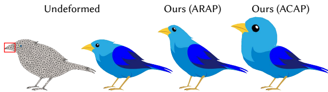
Figure 10: As-conformal-as-possible (ACAP) energy encourages conformality, thus better preserving the color texture by allowing local scaling, while the as-rigid-as-possible (ARAP) energy favors preserving the rigidity. Here the handle (in blue) is placed around the eye and an affine constraint is added to the red region.
